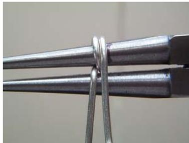
Again, bring the wire up and around the pliers and then down so that the end of the wire is pointing down towards the floor.
