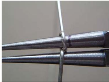
To make the second loop, reposition the first loop back onto the top jaw of the pliers, about the wire lengths from the mark.
