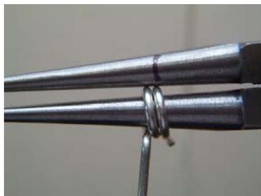
Reposition the wire onto the bottom jaw, and continue pulling the wire around the jaw...
