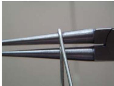
Grab the tip of the wire with your fingers and gently pull it towards you, wrapping the wire around the round nose pliers.
